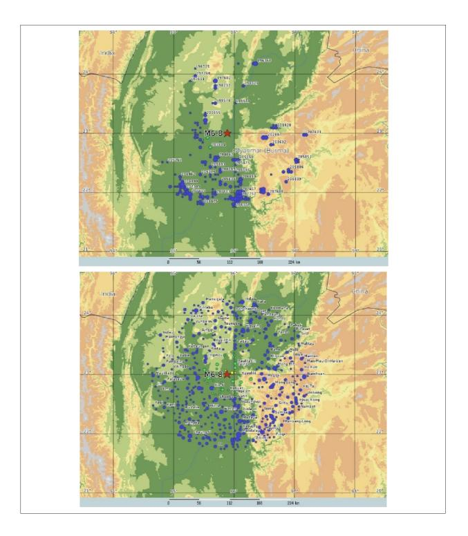
*Figure 10:* Map of calculated mean damage due to the M6.8 earthquake of 11 November 2012 in Myanmar; top LandScan urban data, and bottom QLARM data. The color indicates the mean damage, ranging from blue (minor) to yellow (significant).
